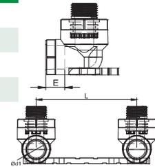
MALE DOUBLE BATTERY CONNECTION- SLAB
