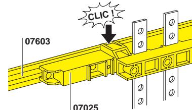
Support 07025 clipped onto Multifix rail.
