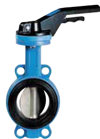
1154 - Disc CF8M / Seat FKM (Viton®) Temperature range: -5°C/+180°C.
