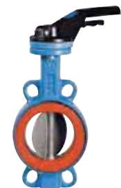
1157 - Disc CF8M / Seat Silicone Temperature range: -30°C/+150°C.
