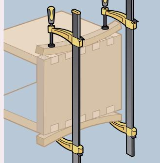
**TIP 4** Tighten the clamps progressively. Depending on the complexity of the job you could be working with four, or even eight bar clamps at the same time, so your aim is to bring all the joints together at the same moment, without any undue stress to the job.
