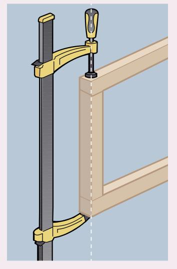
**TIP 3** When clamping up wide carcasses put a rigid piece of wood between the clamping pads. It's even better if the wood is slightly convex, because this will spread the effect of the clamp more evenly across the joint and ensure a better finish. To do this you need at least three hands so hold the two pieces of wood in position with a small 'C' or 'F' clamp leaving both hands free to accurately position the large bar clamps.
