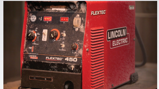
Among other tests, the Flextec™ 450 was subjected to extreme temperature environmental testing, including heat, cold, humidity, rain and dust.
